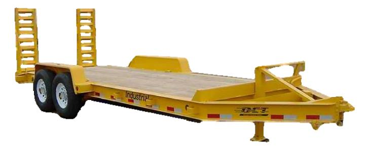
8" I-Beam Frame Chain Tray Choice of Ramps Torsion Axles L.E.D. Lights Low Deck Height
