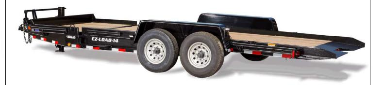
*Features:* Torsion Axles L.E.D. Lights Treated Wood Floor Rubrail & Stakepockets
